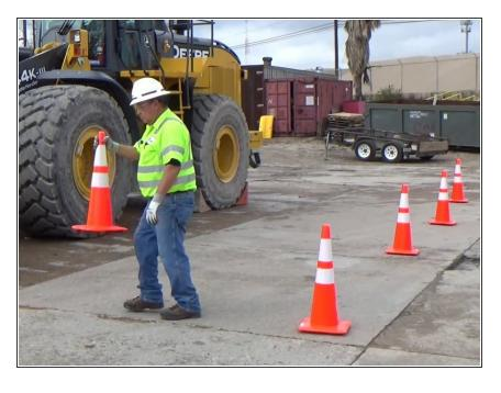
Use safety cones to mark a perimeter around the machine.
