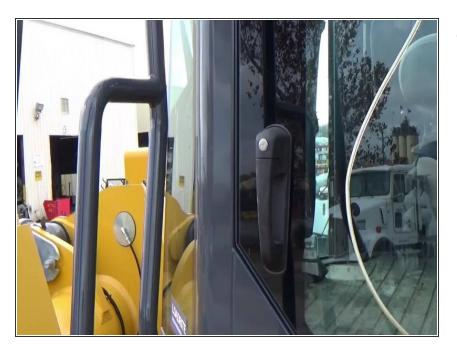
Wrap the lockout cable from the door handle to the hand-rail.
