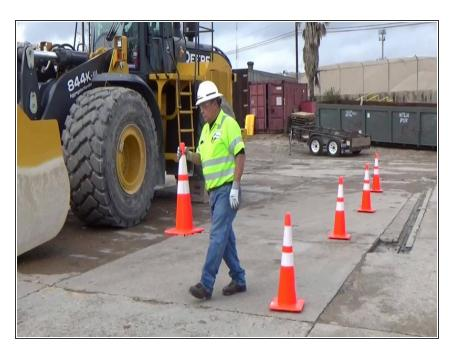
Ensure a perimeter is set from 10' front to back of the machine.
